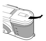
**b** Insert four AA batteries with the **+** and **-** terminals placed as shown.
